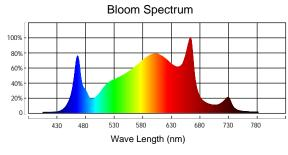
Muizlux Spectra offers continuous spectral photon emission across the PAR 400-700nm wavelength range, balancing energy efficiency with quality of light for desired plant response and human work environment.
